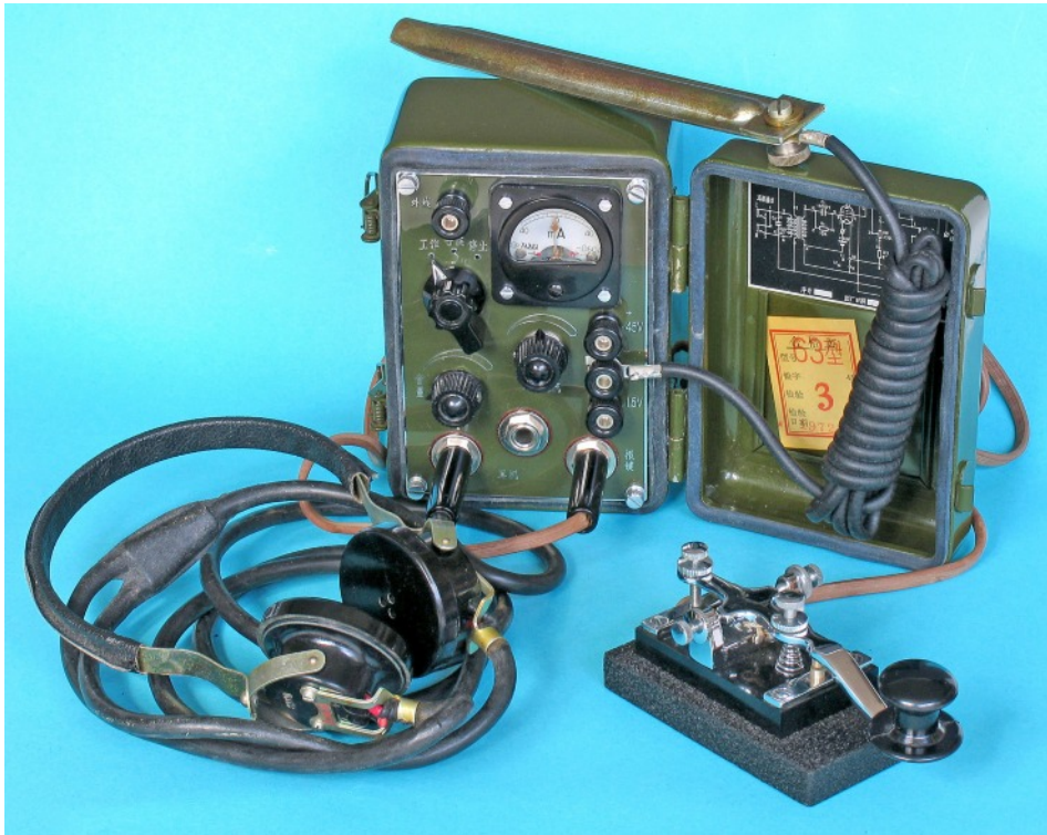
Line telegraph Model 63 with originally issued headphones, earth pin and Morse key.
