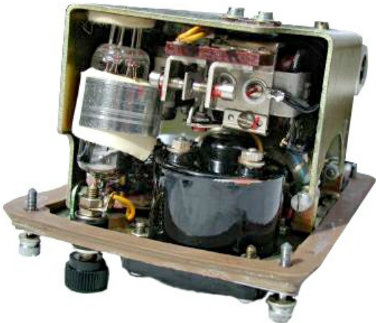
Top view of opened Model 63 showing spare valve, calling relay and line current meter (above).
